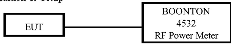
1. The output of the transmitter is connected to the BOONTON RF Power Meter.
