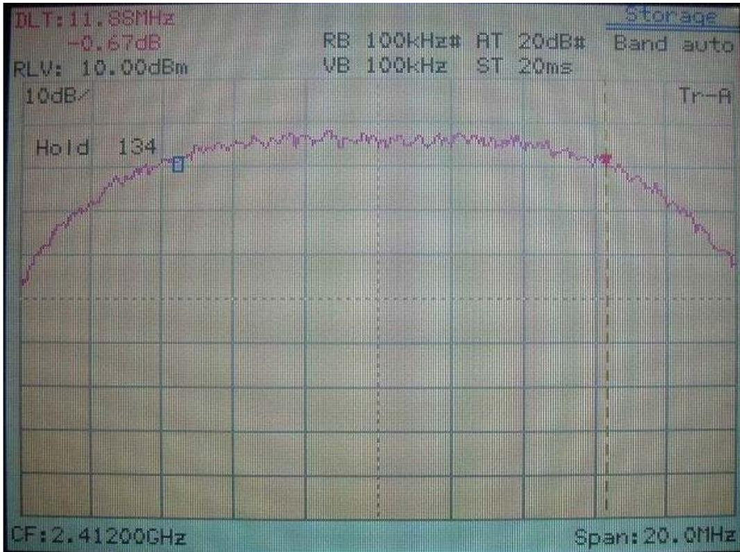
6dB Bandwidth of Channel 6 (The minimum 6dB BW at least 500kHz)
