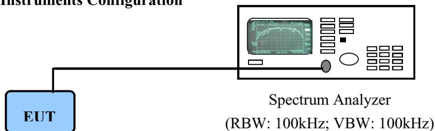
*P.S.: Notebook computer to control the EUT at maximal power output and channel Number and set antenna kit*
