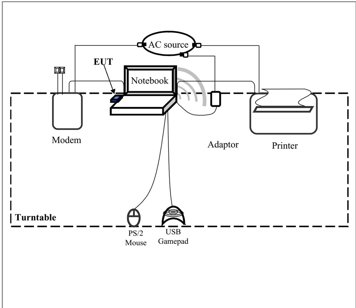
The tests below are carried with the EUT transmitter set at high power in TDD mode. The EUT is forced to select of output power level and channel number by notebook computer.
