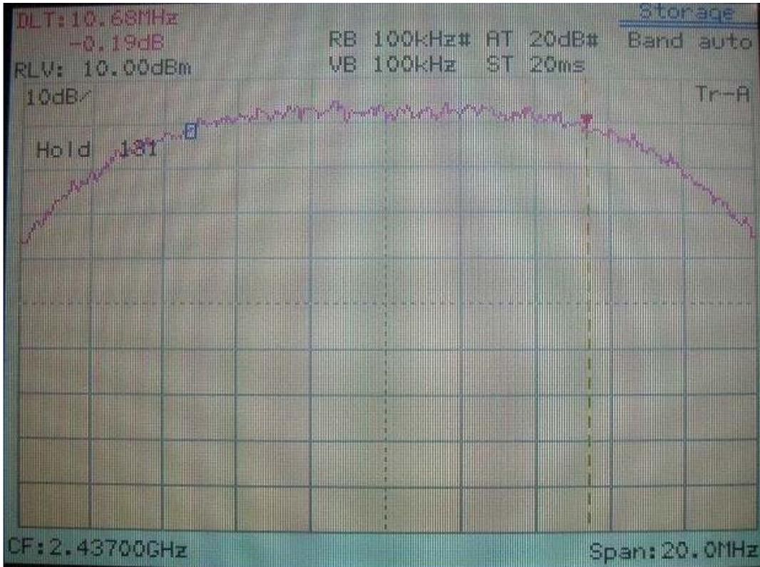
6dB Bandwidth of Channel 11 (The minimum 6dB BW at least 500kHz)
