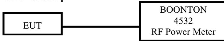
1. The output of the transmitter is connected to the BOONTON RF Power Meter.
