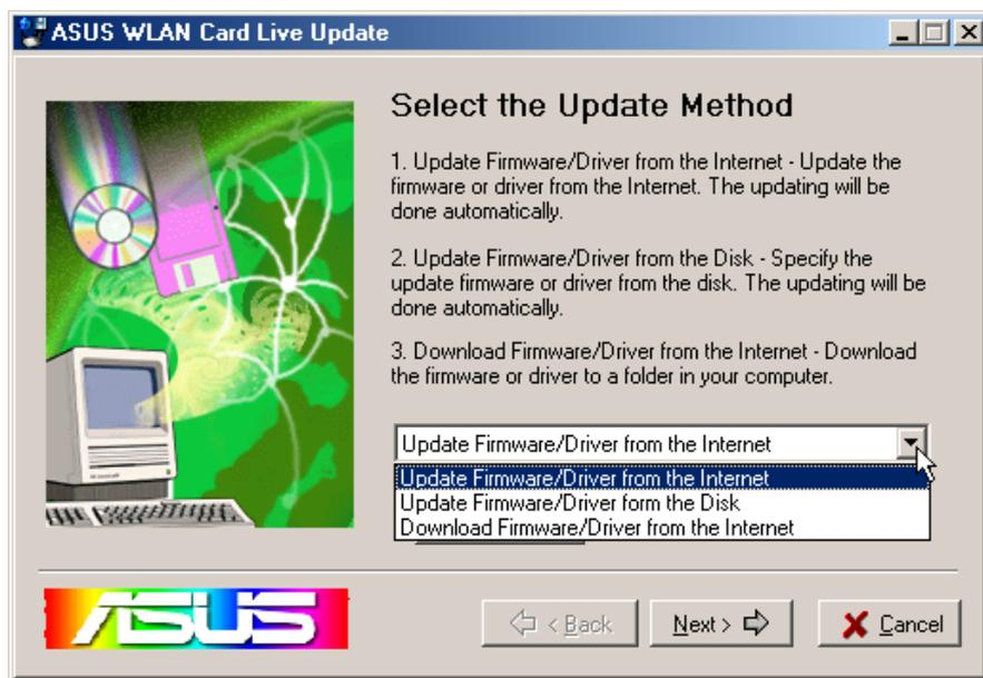
**Update Firmware/Driver from the Internet:** Lets you update the ASUS SpaceLink PC Card's firmware or driver from the Internet. The updating (running the flash utility or the installation program) will be done automatically.
