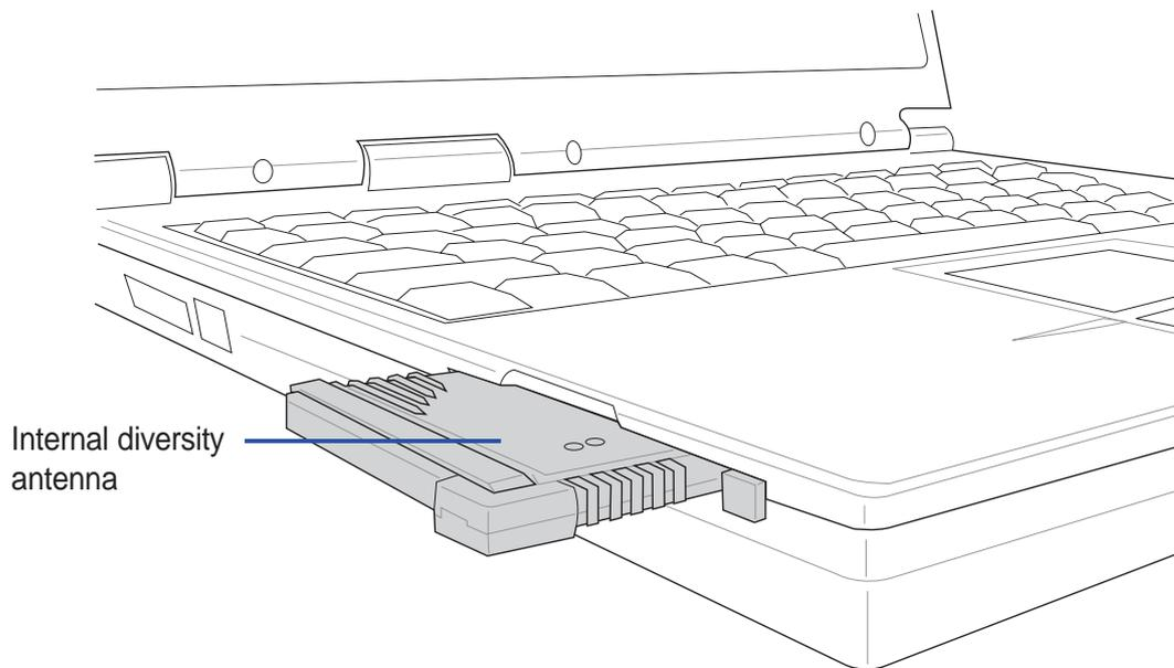
**Inserted ASUS SpaceLink PC Card - Antenna Down**
