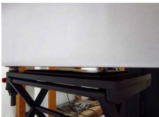
Fig.4 EUT Lap held mode to flat phantom (Test distance is 10.5 mm)
