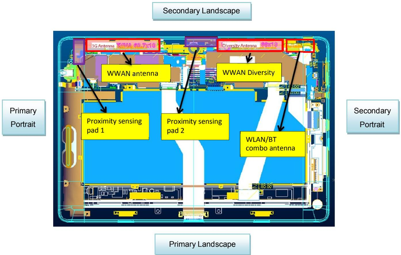
Power reduction applied for each wireless mode and orientation
