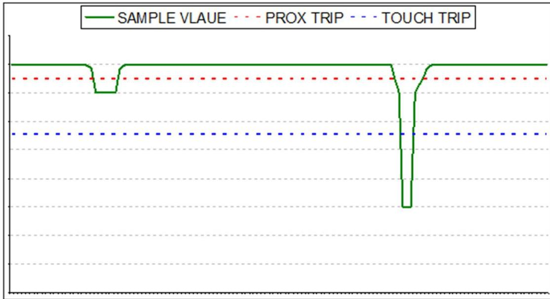
Figure 2.3 Sensing Threshold Filtering
