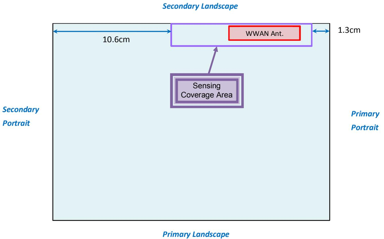
**Figure:** Front face view of coverage area
