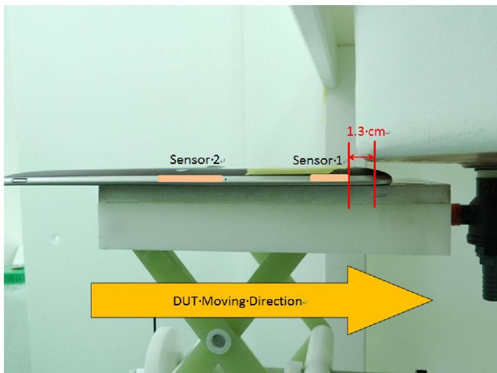
**Figure:** Bottom face distance to edge (First time triggering)
