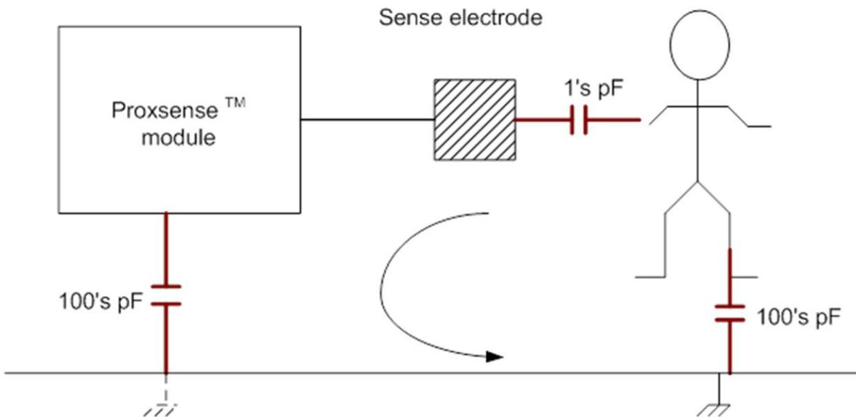
If no physical connection exists between ground and the ProxSense module, improve coupling by using a large ground plane. Electrically connected devices have better PROXIMITY and TOUCH sensitivity.
