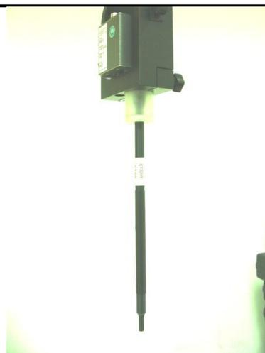
Fig 5.2 Photo of ET3DV6/ET3DV6R
