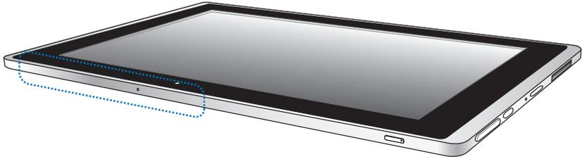
1. The 3G antenna is placed on the top side of your ASUS Transformer Pad.
