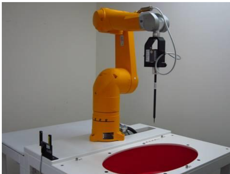
Fig.1 Photograph of the SAR measurement system
