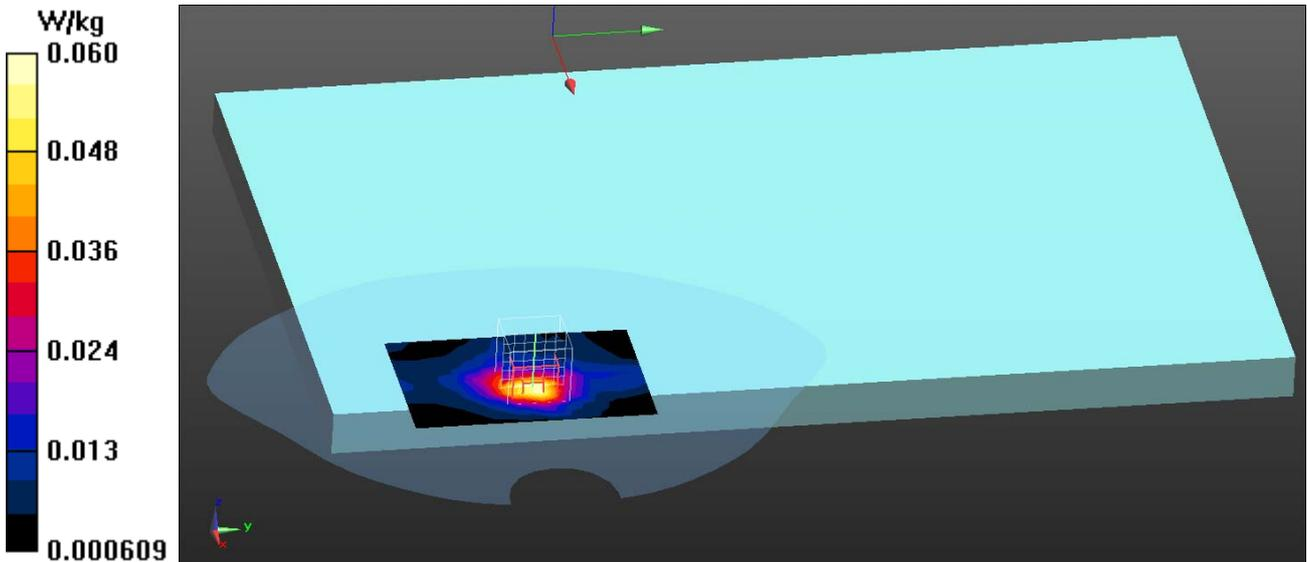
802.11b Aux Antenna EUT Back Z-Axis plot
