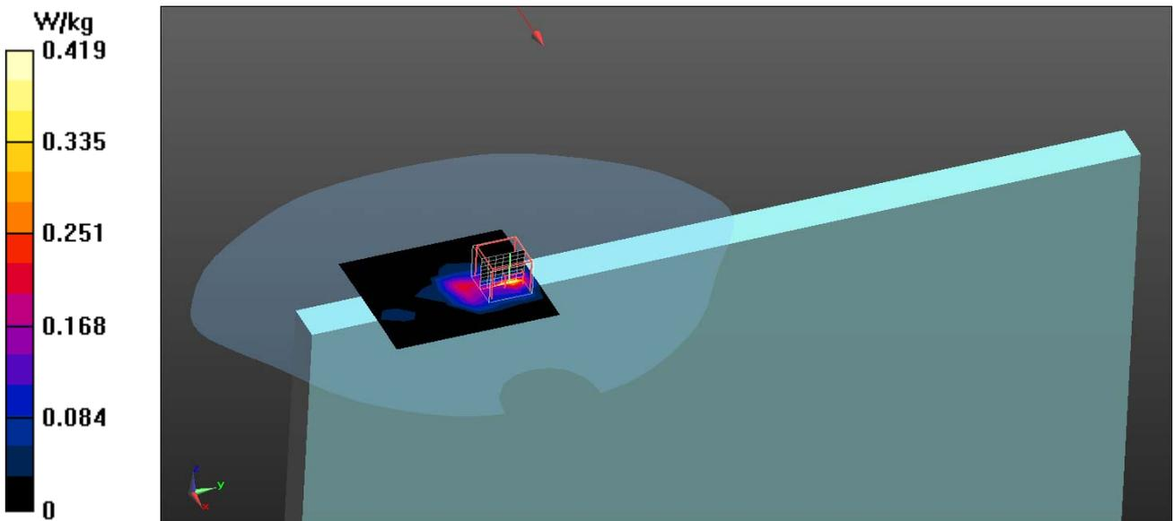
802.11a Main Antenna EUT Top Z-Axis plot
