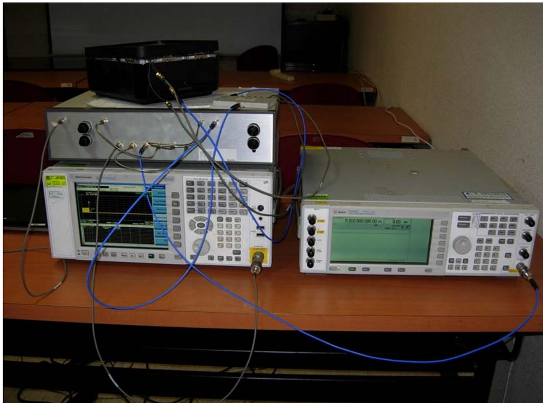
**DFS Set-up Photo: Master and Slave(UUT)**
