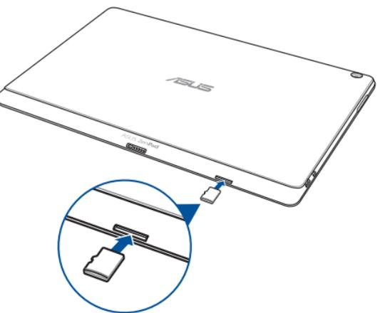
**NOTE:** The memory card slot supports microSD, microSDHC, and microSDXC card formats.
