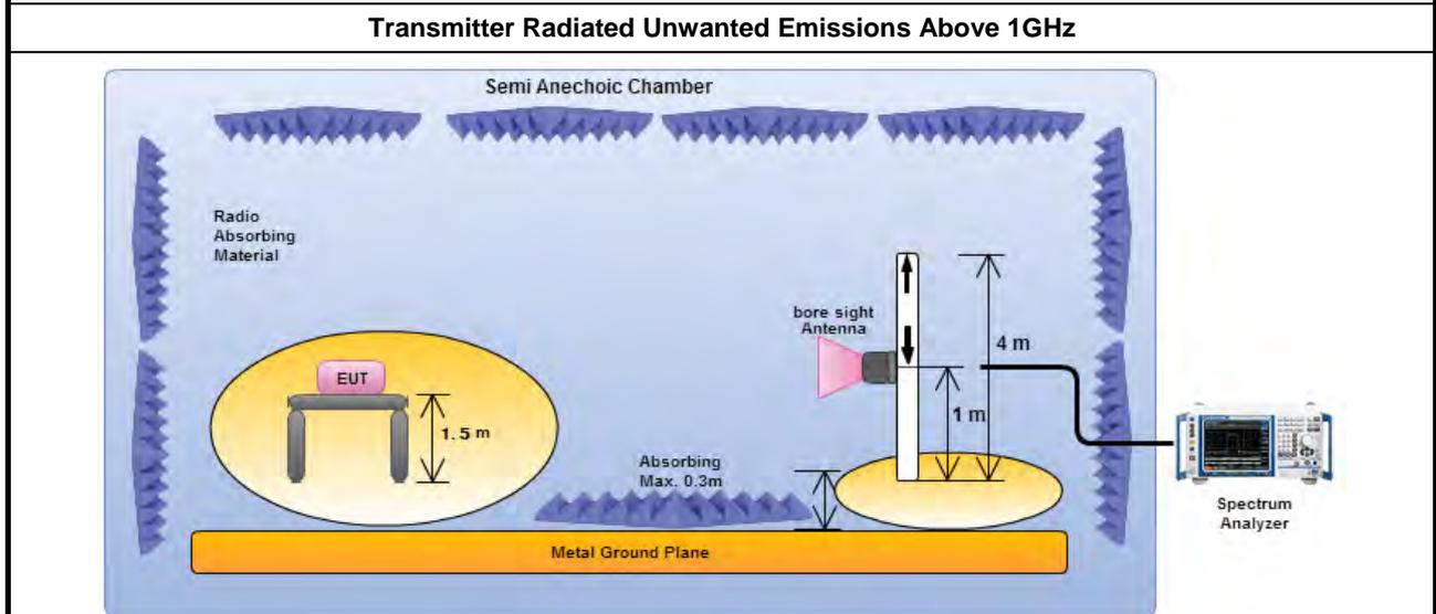
Electric field tests shall be performed in the frequency range of 1 GHz to 10th harmonic of highest fundamental frequency or 40 GHz using a calibrated horn antenna.
