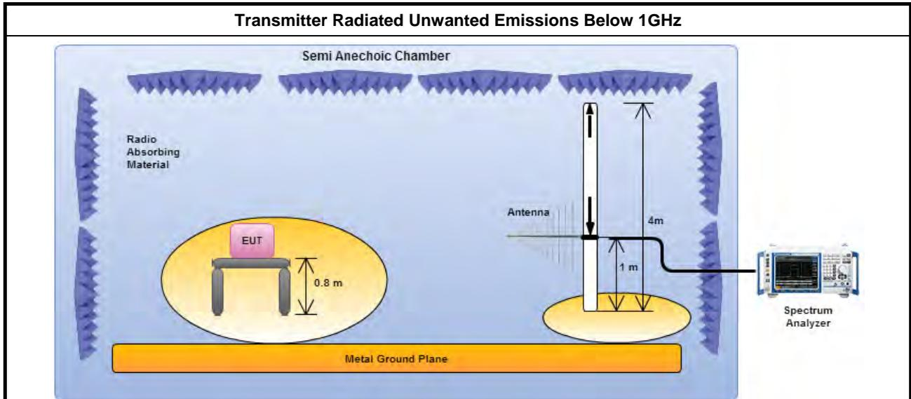
Magnetic field tests shall be performed in the frequency range of 9 kHz to 30 MHz using a calibrated loop antenna. Electric field tests shall be performed in the frequency range of 30 MHz to 1000 MHz using a calibrated bi-log antenna.
