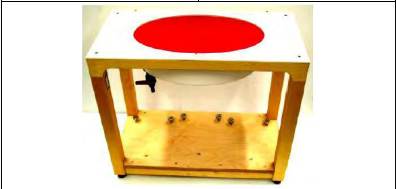
The ELI4 phantom is intended for compliance testing of handheld and body-mounted wireless devices in the frequency range of 30 MHz to 6 GHz. ELI4 is fully compatible with standard and all known tissue simulating liquids.
