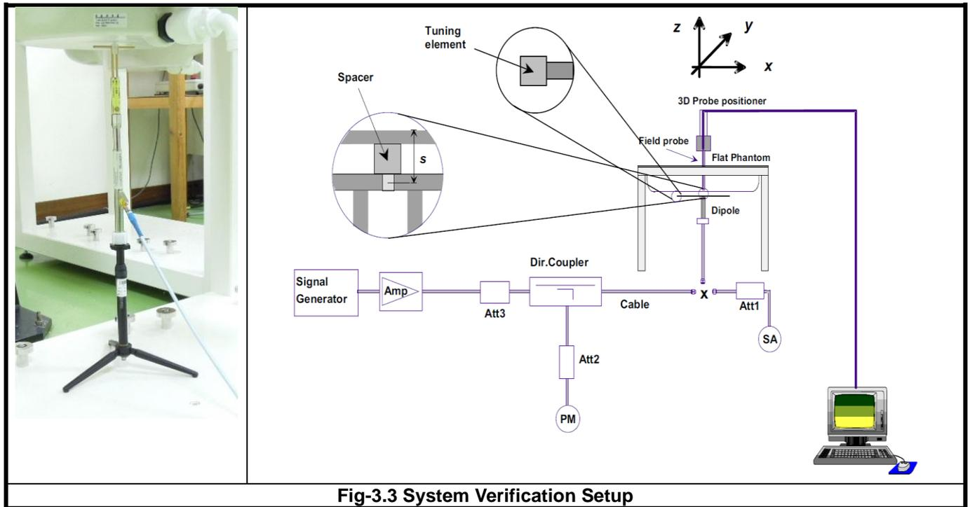
**Fig-3.3 System Verification Setup**
