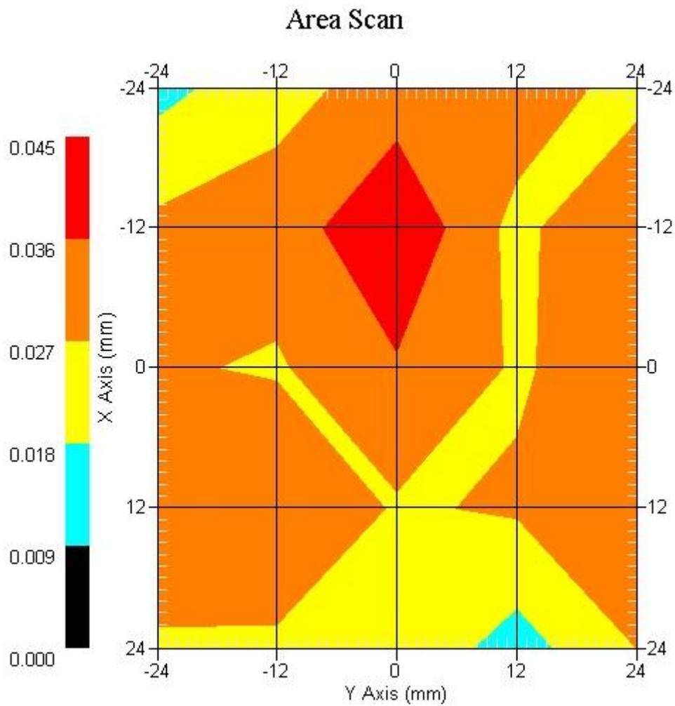
802.11g- Yageo, Tx1 Antenna, EUT Back Z-Axis plot
