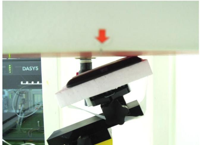
**Rear Face of EUT with 0 cm Gap
