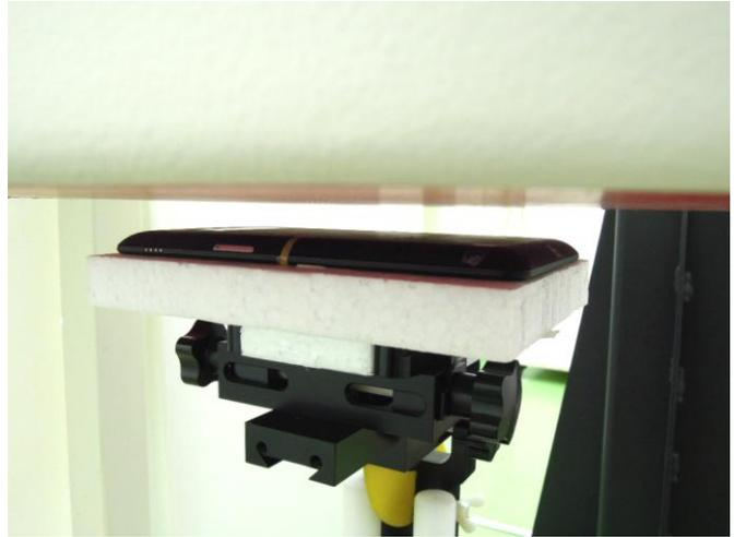
Rear Face of EUT with 1.4 cm Gap
