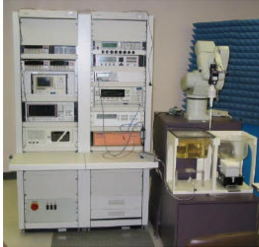
The ALIDX-500 Dosimetric SAR Measurement System was developed jointly with APREL Laboratories and IDX Robotics for use within wireless development and the compliance environment. The system consists of a six axis articulated arm, and controller for precise probe positioning (0.05 mm repeatability). Custom software has been developed to enable communications between the robot controller software and the host operating system.
