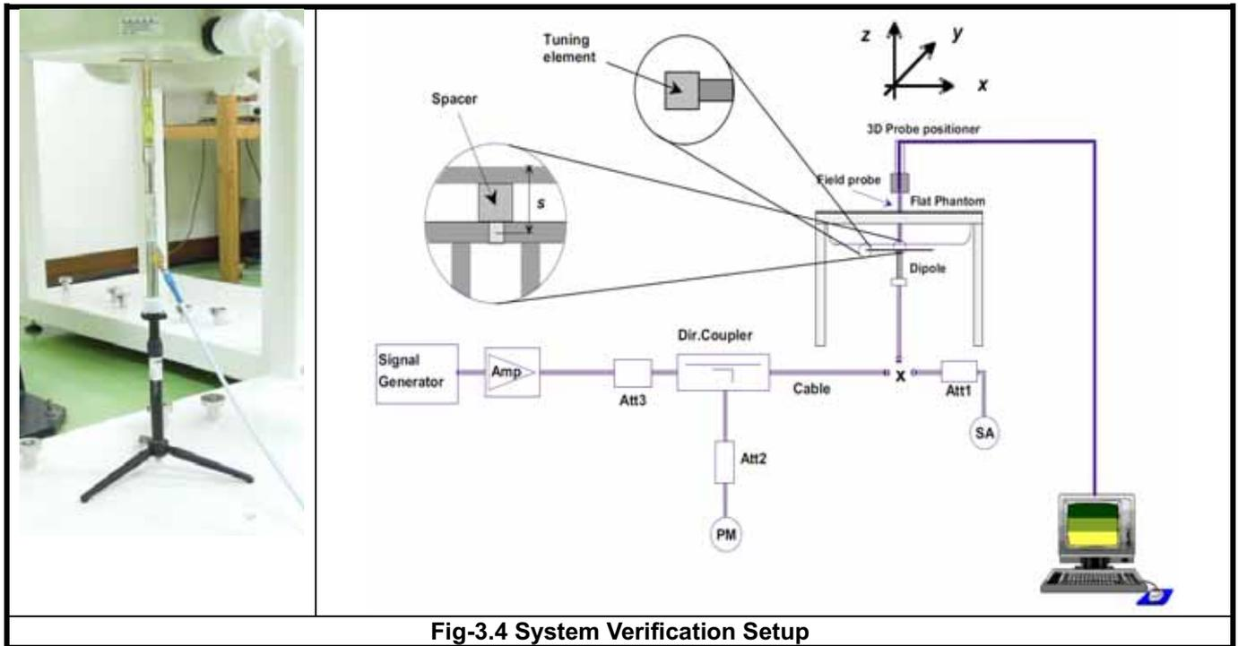
**Fig-3.4 System Verification Setup**
