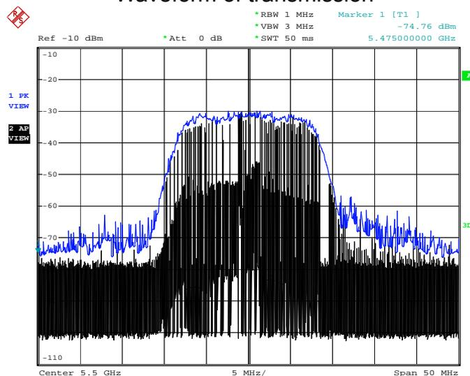
3) Radar signal 1 is applied to the Master device and WiFi traffic signal stop immediately.
