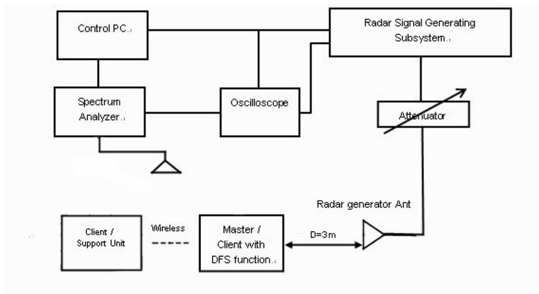
The test transmission will always be from the Master Device to the Client Device. While the Client device is set up to associate with the Master device and play the MPEG file (6  $\frac{1}{2}$  Magic Hours) from Master device, the designated MPEG test file and instructions are located at:
