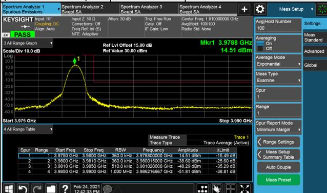
**Channel 664332 (3964.98MHz) QPSK 1 RB / 77 RB Offset**
