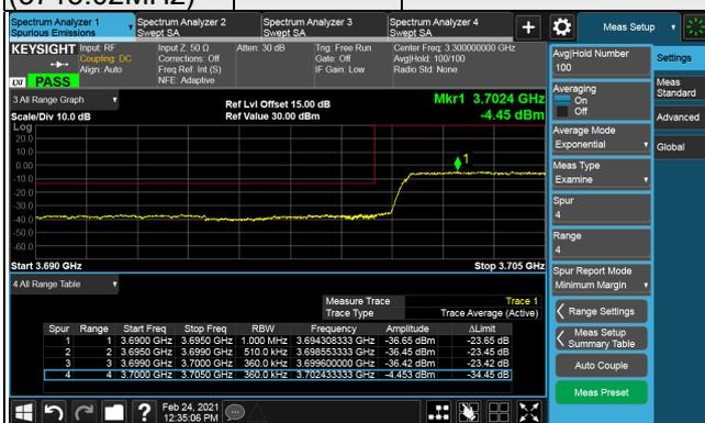
**Channel 647668 (3715.02MHz) QPSK 78 RB / 0 RB Offset**
