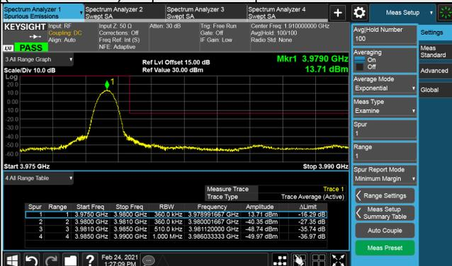
Channel 648668 (3730.02MHz) QPSK 162 RB / 0 RB Offset
