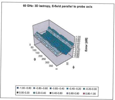
Probe isotropy for  $E_{tot}$ : probe rotated  $\phi=0^\circ$  to 360°, tilted from field propagation direction  $\vec{k}$  Parallel to the field propagation ( $\psi=0^\circ$  - 90°) at 30 GHz: deviation within  $\pm$  0.30 dB Parallel to the field propagation ( $\psi=0^\circ$  - 90°) at 60 GHz: deviation within  $\pm$  0.38 dB
