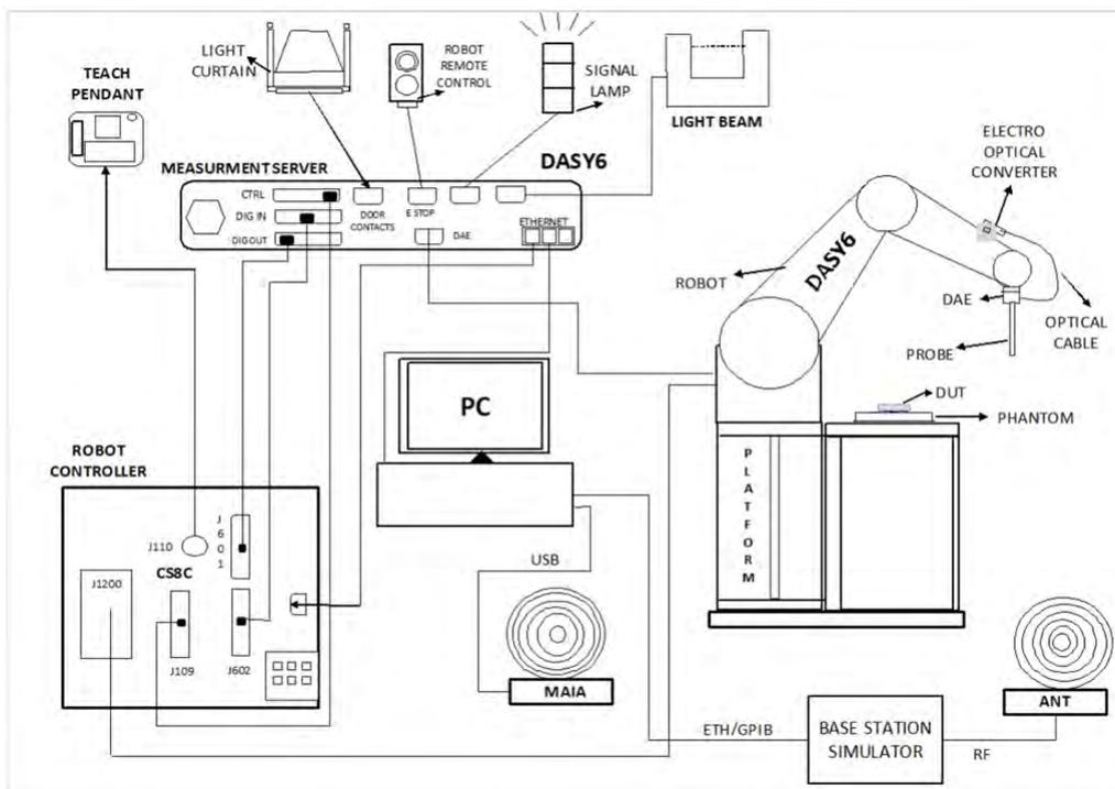
**Fig-3.1 SPEAG DASY6 System Configuration**
