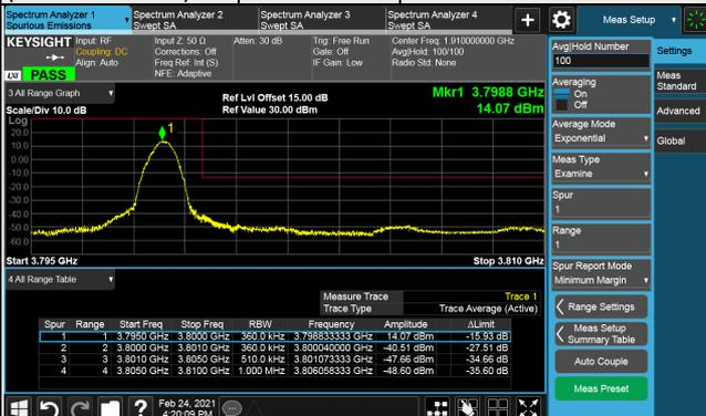
**Channel 651000 (3765.00MHz) QPSK 1 RB / 188 RB Offset**
