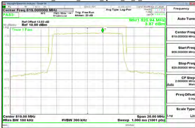
Band30 5MHz_QPSK 1 0 CH27685
