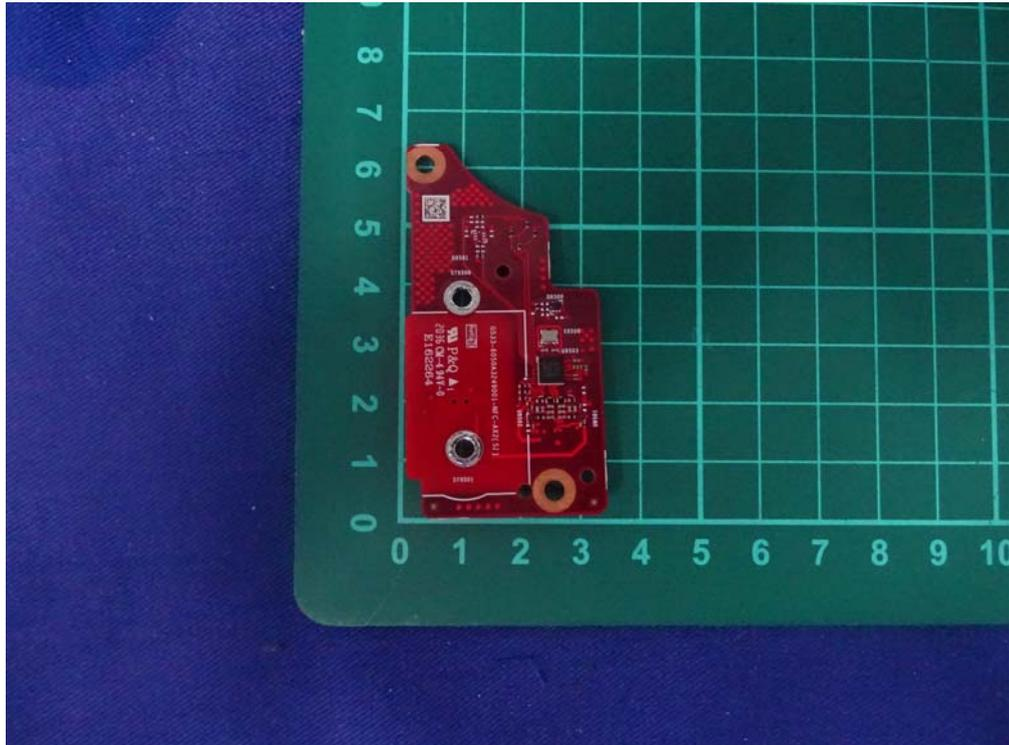
(27) EUT Photo (NFC PCB Board)
