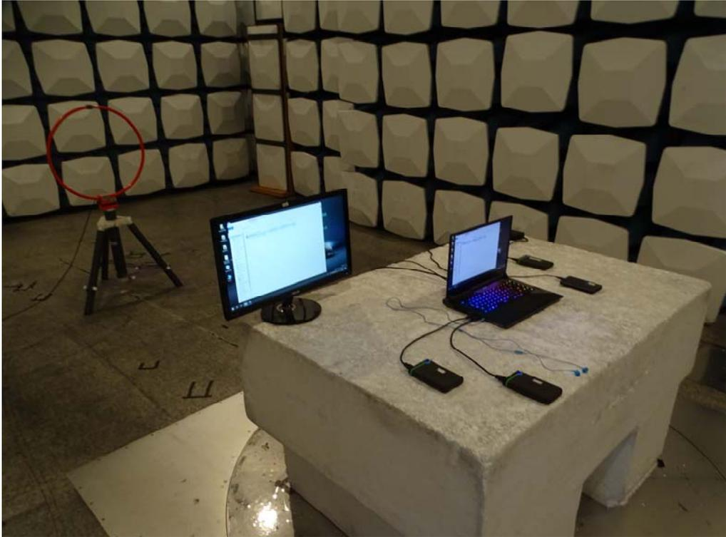
Back View of Radiated Test-LOOP
