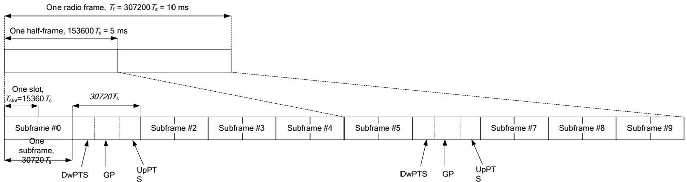
**3GPP TS 36.211 Figure 4.2-1: Frame Structure Type 2**
