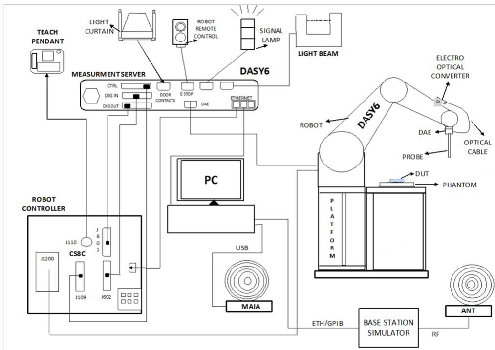
**Fig-3.1 SPEAG DASY6 System Configuration**
