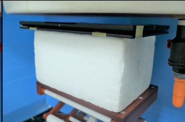
Rear Face of Tablet Mode Tested at 20 mm
