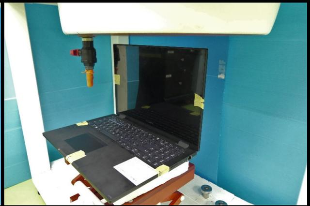
**Top Side of Panel Tested at 25 mm**
