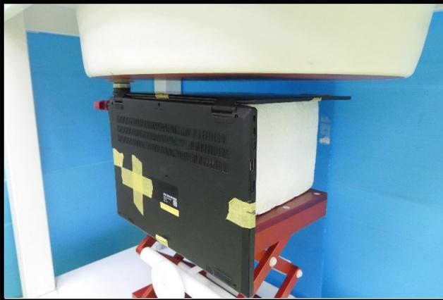
**Back Side of Panel Tested at 25 mm**
