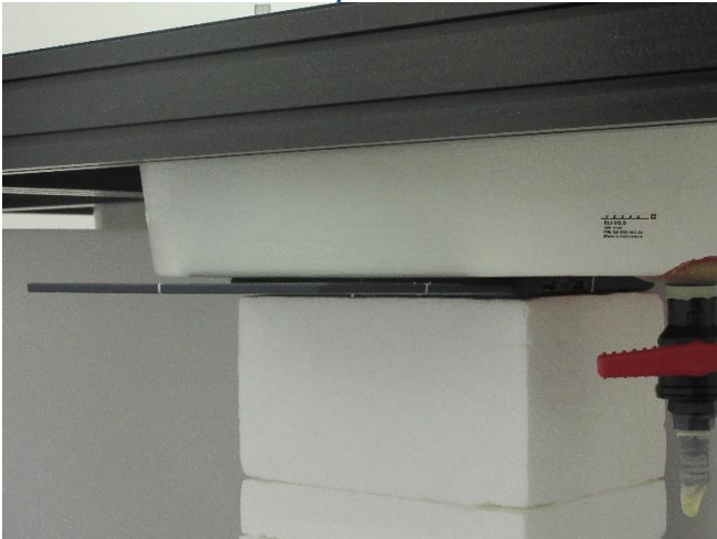
Testing Setup for Extremity, Top Side of Keyboard at 0 mm, Sample 1 & 2
