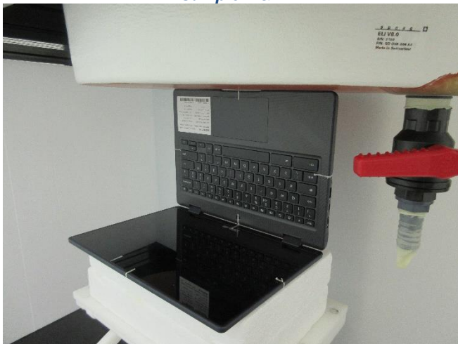
Testing Setup for Body, Front Edge of Laptop at 0 mm, Sample 1 & 2
