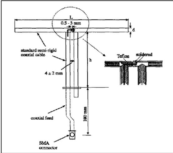
The dipoles used is based on the IEEE-1528 standard, and is complied with mechanical and electrical specifications in line with the requirements of both IEEE and FCC Supplement C. the table below provides details for the mechanical and electrical specifications for the dipoles.
