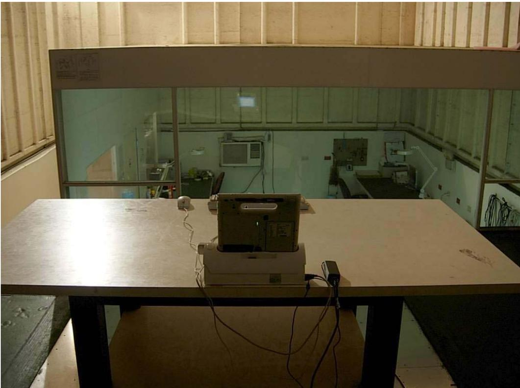
Front View of Radiated Test (above 30MHz)
