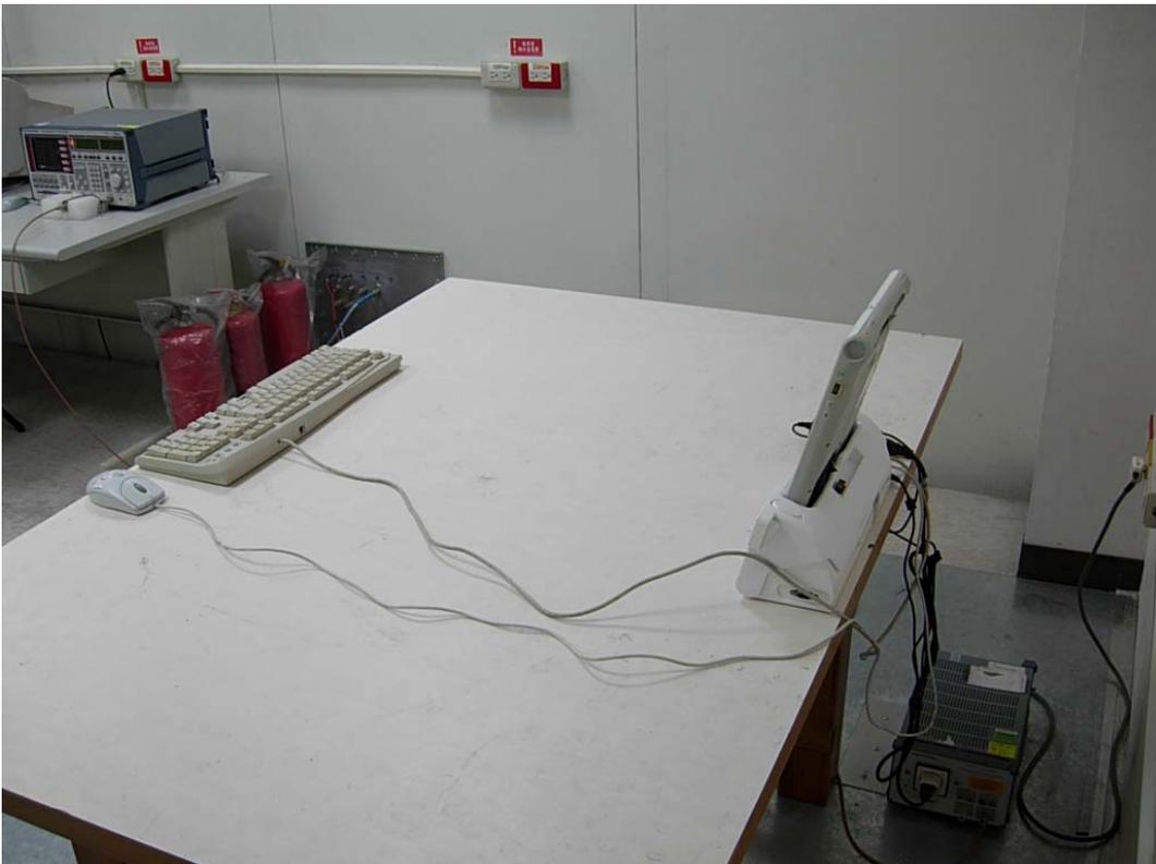
Front View of Radiated Test (below 30MHz)
