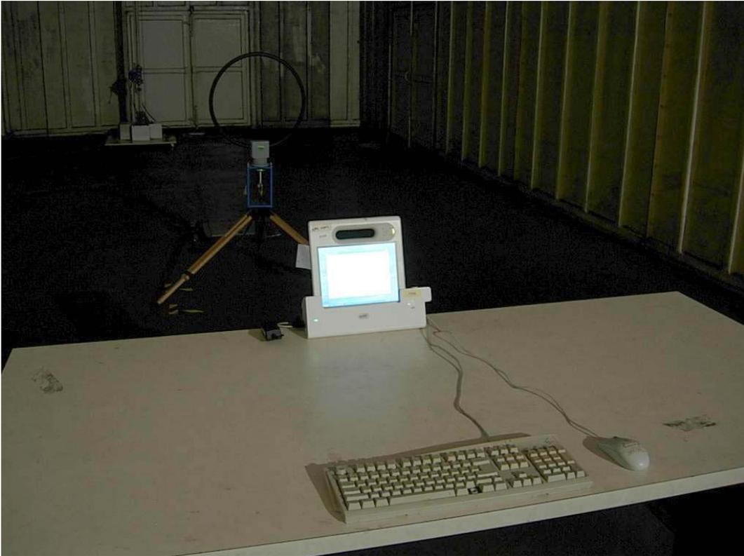
Back View of Radiated Test (below 30MHz)
