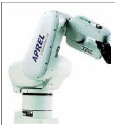
ALSAS-10U utilizes a six axis articulated robot, which is controlled using a Pentium based real-time movement controller. The movement kinematics engine utilizes proprietary (Thermo CRS) interpolation and extrapolation algorithms, which allow full freedom of movement for each of the six joints within the working envelope. Utilization of joint 6 allows for full probe rotation with a tolerance better than 0.05mm around the central axis.
