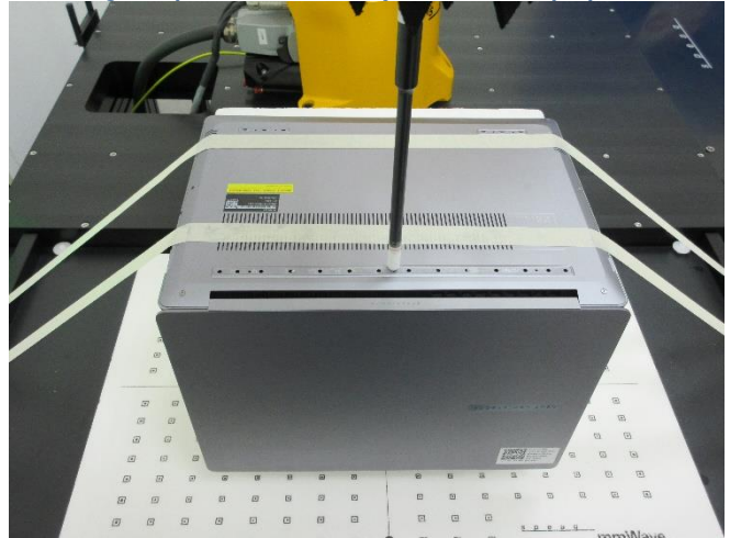
Testing Setup for Power Density, Bottom of Laptop at 2 mm
