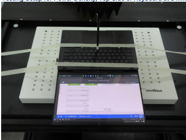
Testing Setup for Power Density, Top Side of Keyboard at 2 mm
