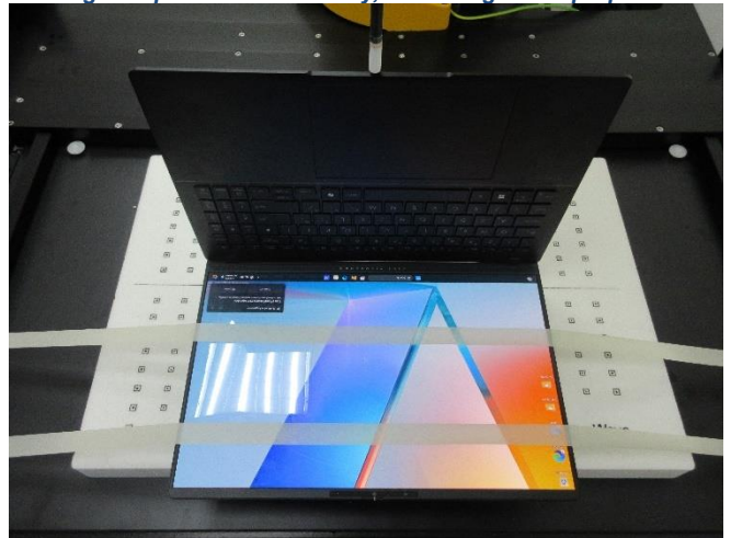
Testing Setup for Power Density, Front Edge of Laptop at 2 mm
