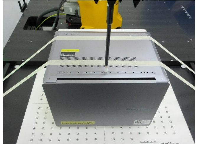
Testing Setup for Power Density, Bottom of Laptop at 0 mm
