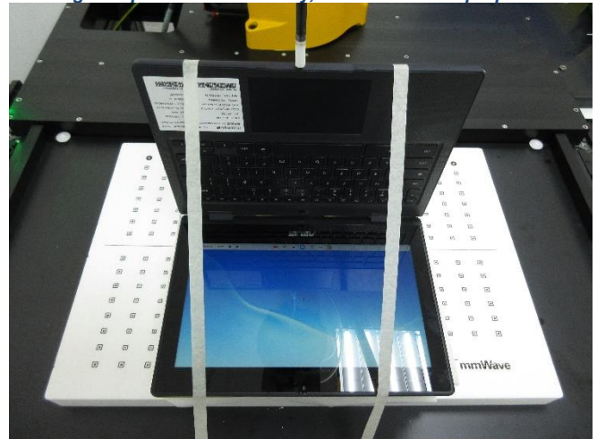
Testing Setup for Power Density, Front Side of Laptop at 2 mm
