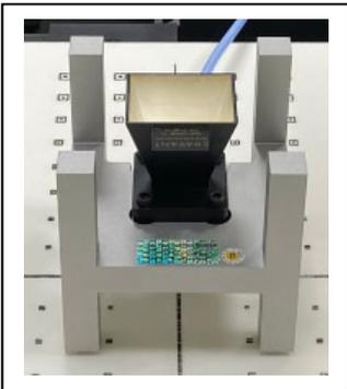
The verification sources apply to system check or verification at specific mmWave frequencies. The sources comprise horn-antennas and very stable signal generators.
