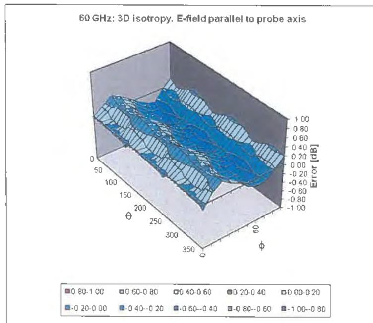
Probe isotropy for  $E_{tot}$ : probe rotated  $\phi = 0^\circ$  to  $360^\circ$ , tilted from field propagation direction  $\hat{k}$
