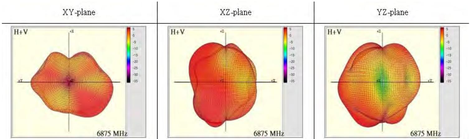
Max Antenna 3D Radiation Pattern 6875-7125 MHz
