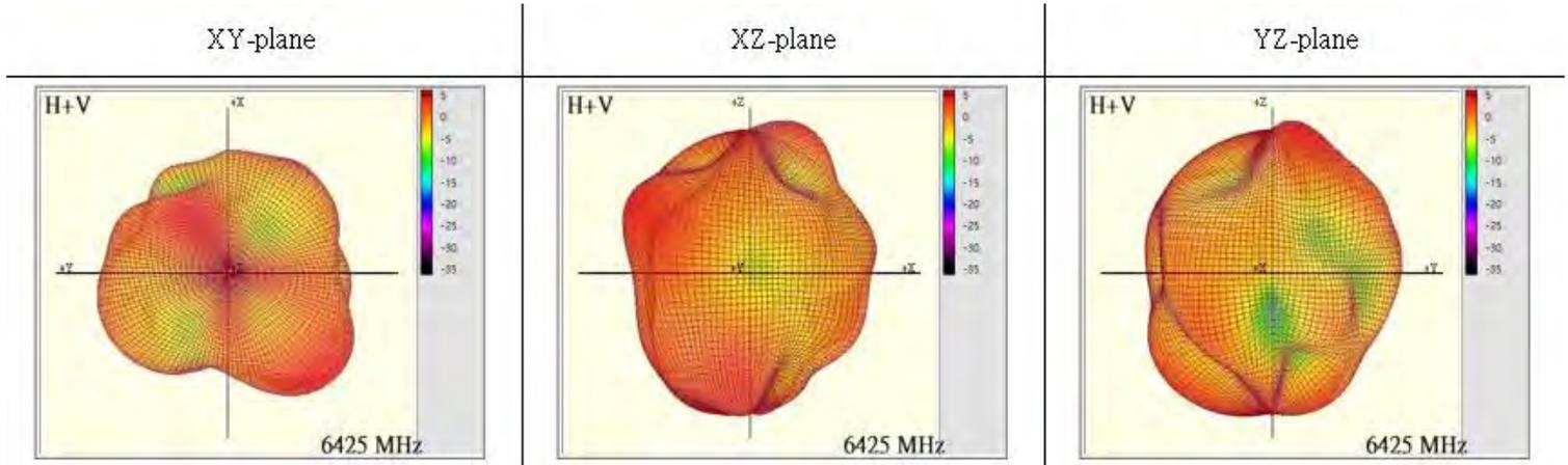
Max Antenna 3D Radiation Pattern 6525-6875 MHz
