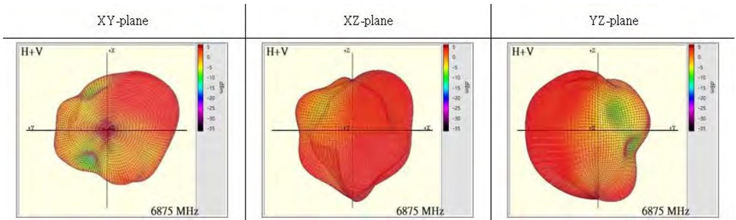
Max Antenna 3D Radiation Pattern 6875-7125 MHz
