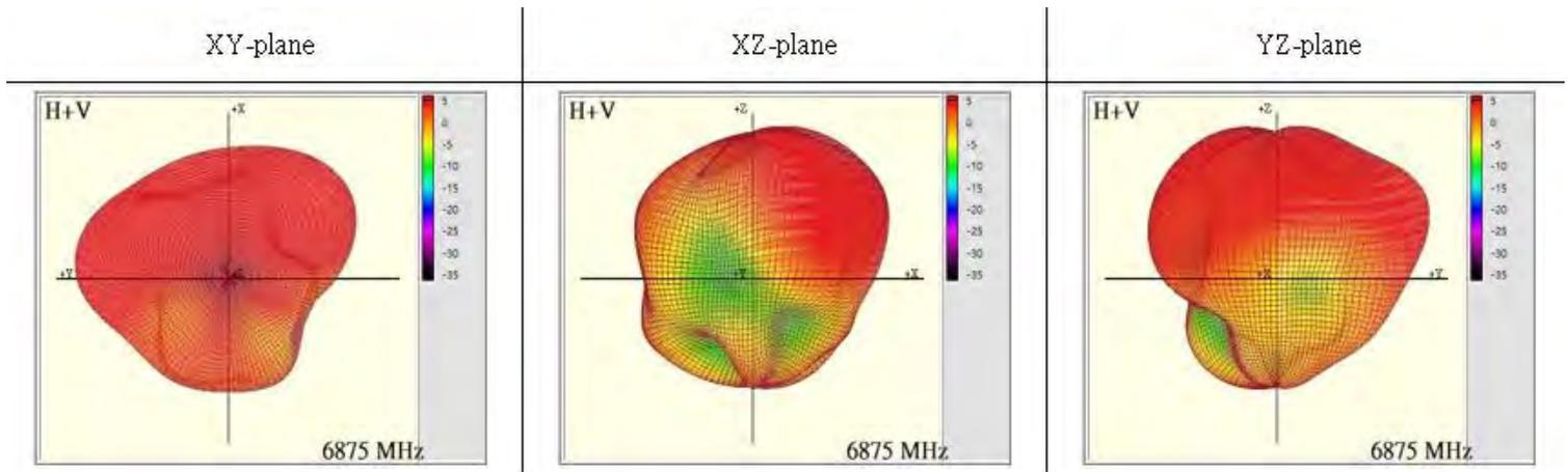
Max Antenna 3D Radiation Pattern 6875-7125 MHz
