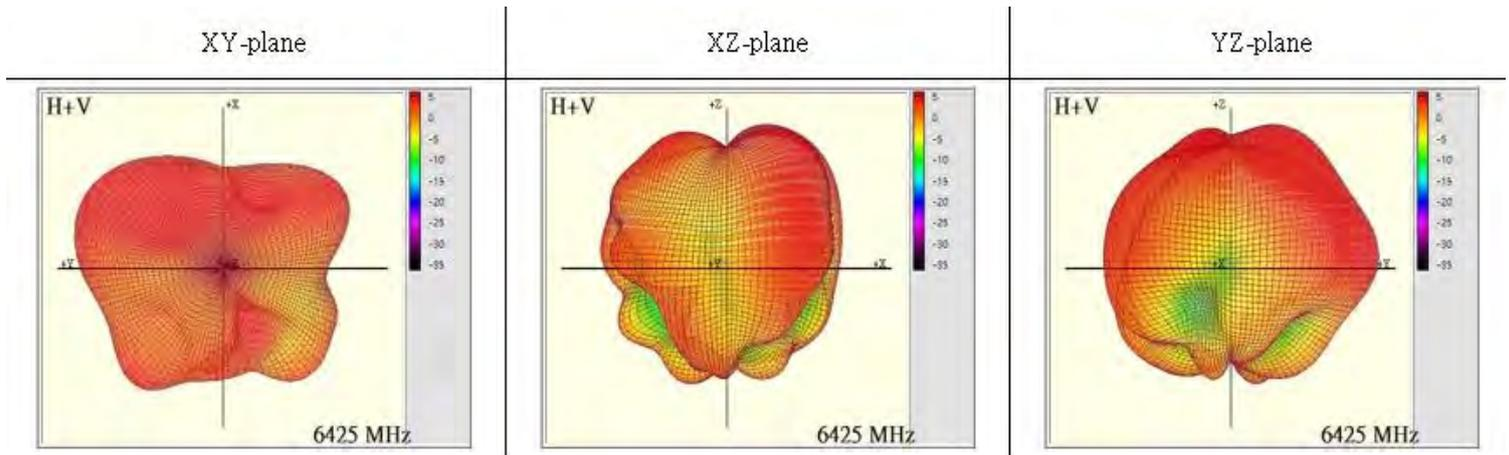
Max Antenna 3D Radiation Pattern 6525-6875 MHz
