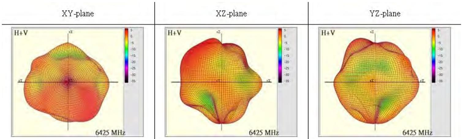
Max Antenna 3D Radiation Pattern 6525-6875 MHz
