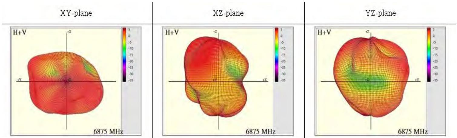
Max Antenna 3D Radiation Pattern 6875-7125 MHz
