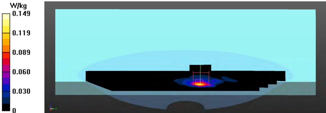
**802.11b EUT Bottom(NB) (PULSE Main Antenna) Z-Axis plot**
