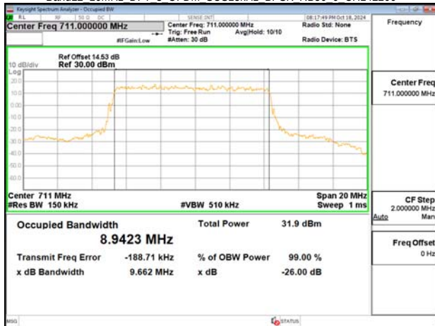
Band12 10MHz DFT s OFDM SCS15kHz BPSK RB50 0 CH142200
