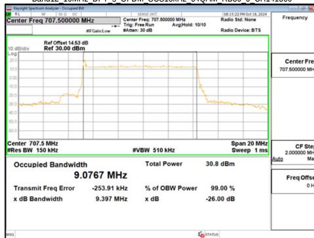
Band12 10MHz DFT s OFDM SCS15kHz 64QAM RB50 0 CH142200
