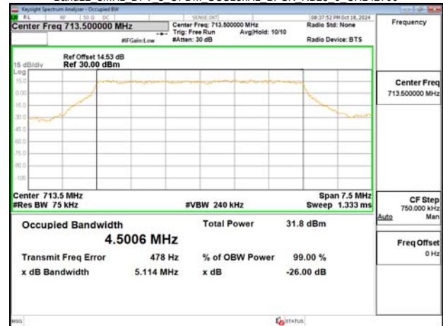
Band12 5MHz DFT s OFDM SCS15kHz BPSK RB25 0 CH142700
