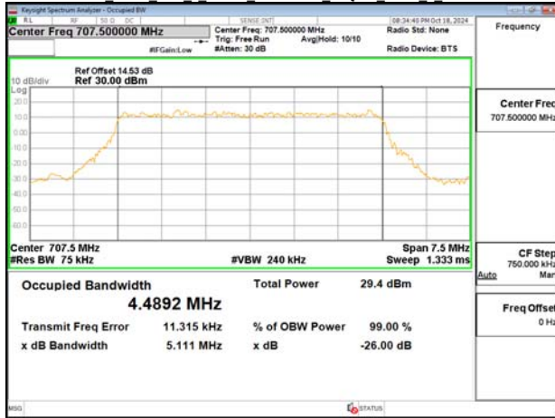
Band12 5MHz DFT s OFDM SCS15kHz 64QAM RB25 0 CH142700
