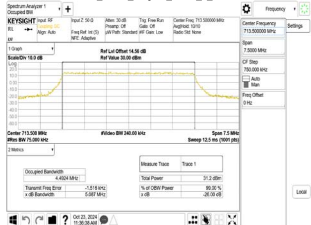
Band12_5MHz_16QAM_RB25_0_CH23155
