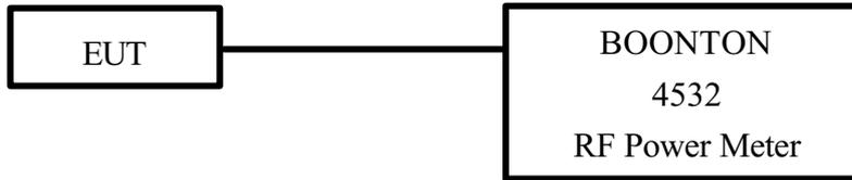
1. The output of the transmitter is connected to the BOONTON RF Power Meter.
