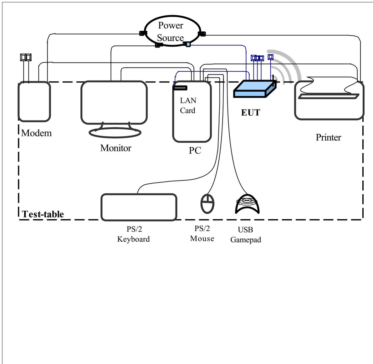
The tests below are carried with the EUT transmitter set at high power in TDD mode. The EUT is forced to select of output power level and channel number by LAN port.
