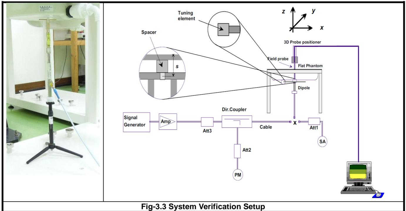
**Fig-3.3 System Verification Setup**
