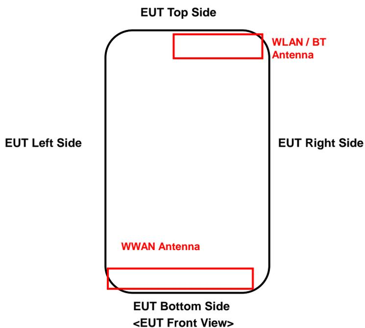
The separation distance for antenna to edge:
