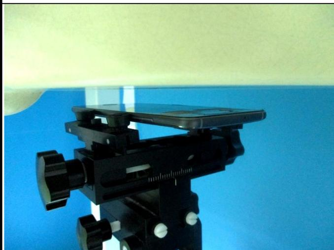
**Front Face of EUT with 1.5 cm Gap**
