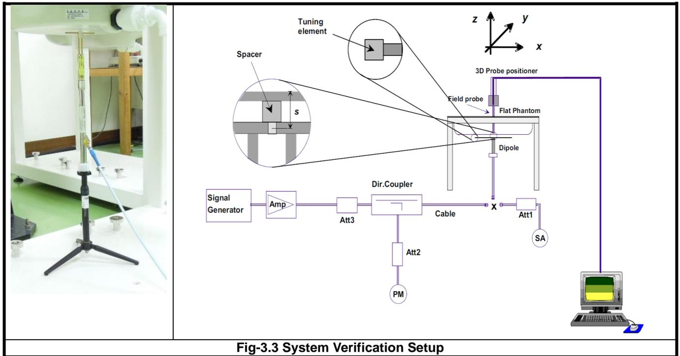
**Fig-3.3 System Verification Setup**
