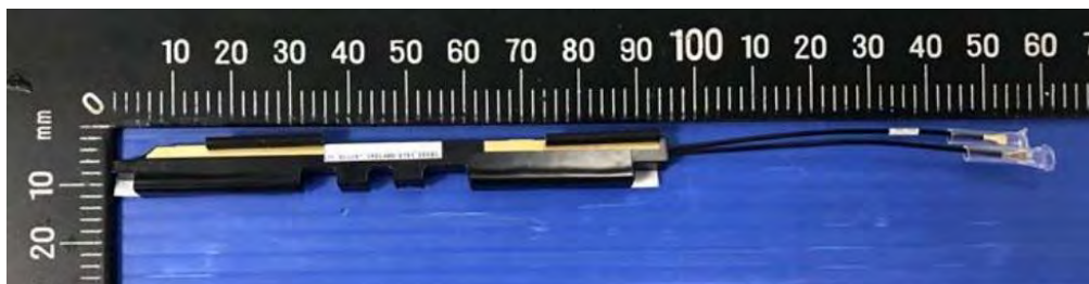
LUXSHARE Main Aux Antenna Vendor LA9RF143-CS-H (MAIN and Aux) ASUS 14008-03280100 (MAIN and Aux)
